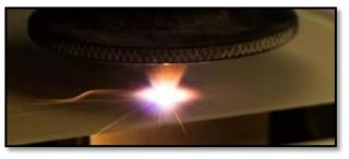
motion control system, moving the substrate below the fixed beam assembly at speeds as fast as 10 in./sec, or faster. Each pulse of the Laser provides an efficient and effective evacuation of molten and ablated ceramic substrate particulates. Well executed scribes allow for subsequent controlled breaks or "snapping" of the substrate to the final size.
